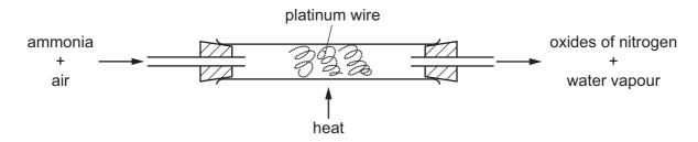
The platinum is chemically unchanged at the end of the reaction.
